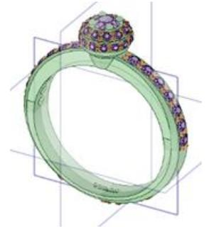
3. **Simulation of the model for the client** – after the initial sketch is ready, the design is saved in a special file, which will allow a simulation to read it. The simulation software allows us to simulate for the client how the ring will be in real life.
