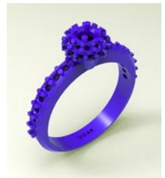
5. **Casting** – after we got our digital 3D polymeric model, we can cast it to the wanted metal. This model is heated in a special plate, into to which the wanted metal is casted. After it has cooled down, we take the metal out of the plate and we get the wanted metal model, which is almost ready.
